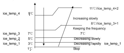
When Tpg\_indoor  $\langle$  ice\_temp\_1, the frequency of the compressor decreases at the speed of 1HZ/1second.
