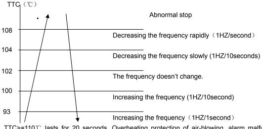
TTC>=110  $^\circ\!\!\!C$  lasts for 20 seconds. Overheating protection of air-blowing, alarm malfunction to the indoor, others don't last.
