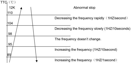
TTC>=110°C lasts for 20 seconds. Overheating protection of air-blowing, alarm malfunction to the indoor, others don't last.
