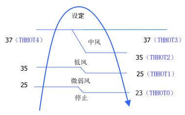
\* Residue heat sending. The indoor fan will send the residue heat at a low speed for 20 seconds. If other conditions are satisfied, when the compressor stops, the indoor system will operate at a light speed. The indoor fan will stop when the coil temperature is below the THHOT0.
