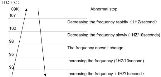
TTC>=110 $^{\circ}$ C lasts for 20 seconds. Overheating protection of air-blowing, alarm malfunction to the indoor, others don't last.
