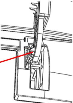
A detailed inset diagram showing the hinge mechanism where the front panel meets the indoor unit's frame. A red arrow from the main diagram points to this inset. |
