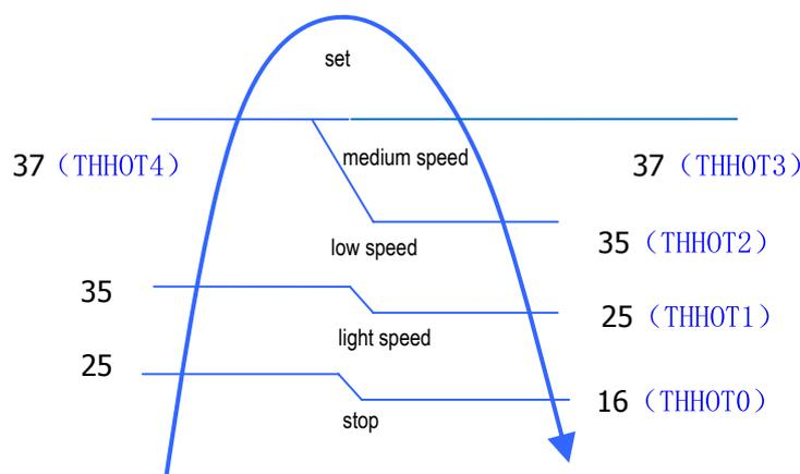
\* Residue heat sending. The indoor fan will send the residue heat at a low speed for 20 seconds.
