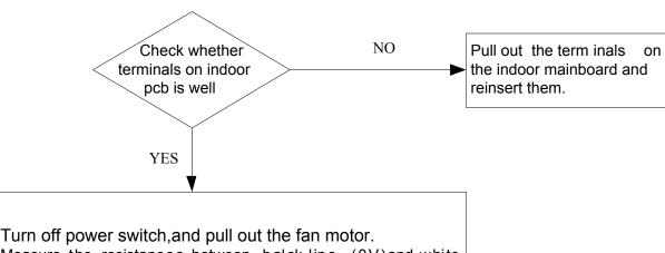
Turn off power switch, and pull out the fan motor. Measure the resistances between balck line (0V) and white line(15V), balck line (0V) and red line(310V) of indoor fan motor.
