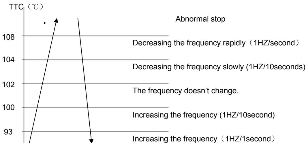
TTC $\geq$ 110°C lasts for 20 seconds. Overheating protection of air-blowing, alarm malfunction to the indoor, others don't last.
