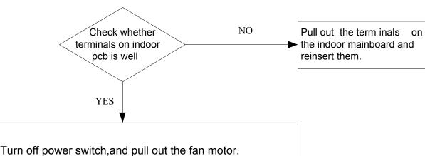
Turn off power switch, and pull out the fan motor.
